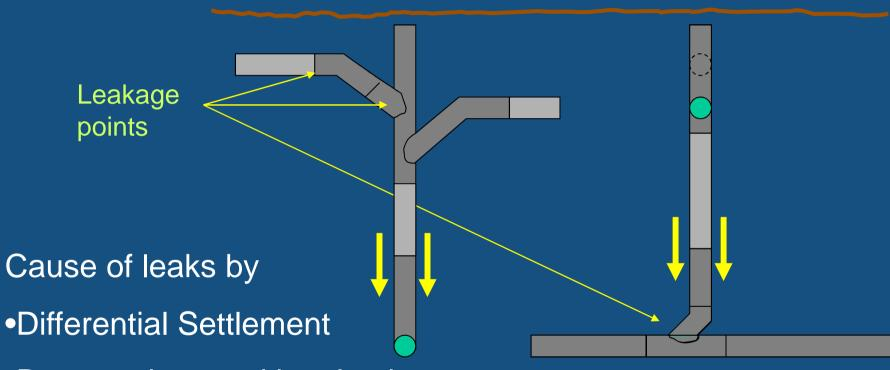
Damaged caused by plumbers making new connections + insufficient bedding and backfill
